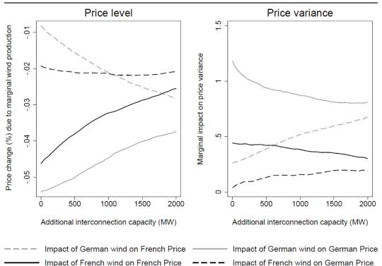
Figure 6: Effect of wind generation when interconnection capacity is increased
