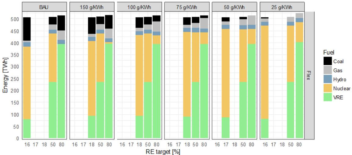
**Figure 5. Evolution of the electricity mix with increasing RE obligations and new sources of flexibility**
