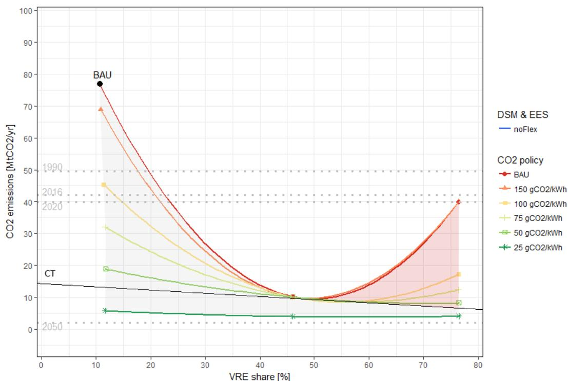
**Figure 3. The performance of total emissions reductions under RE obligations in the system without new sources of flexibility**
