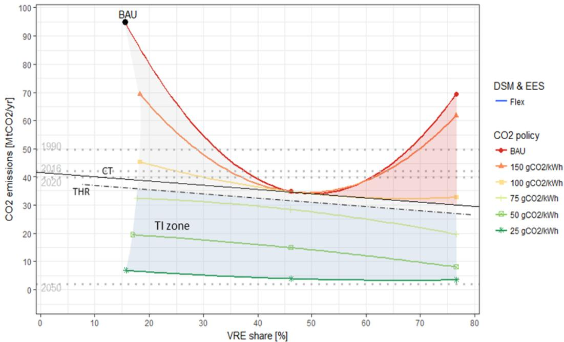
**Figure 6. The performance of total emissions for increasing RE obligation levels in systems with new sources of flexibility**
