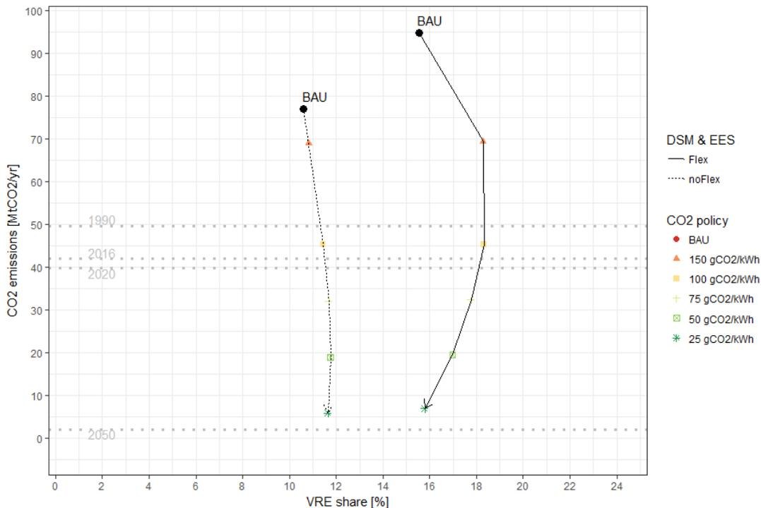
**Figure 1. Optimal share of VRE under different CO2 norms and with/without flexibility in 2050**
