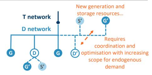
So long as it is well located, generation and storage can offset need for distribution network...
